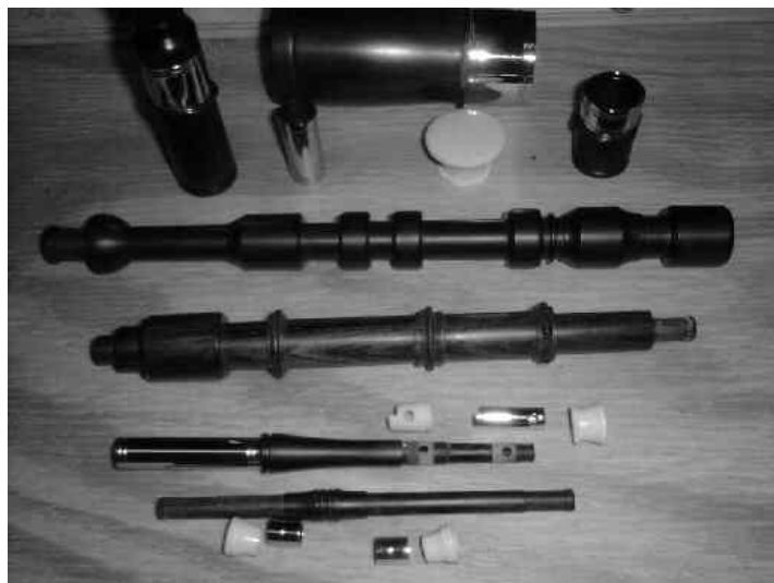
15-Key D set under construction. Chanter is the two pieces in center after turning. Oops, you didn't know extended chanters are often made in two sections? Dang, I let another pipemakers secret slip out!
